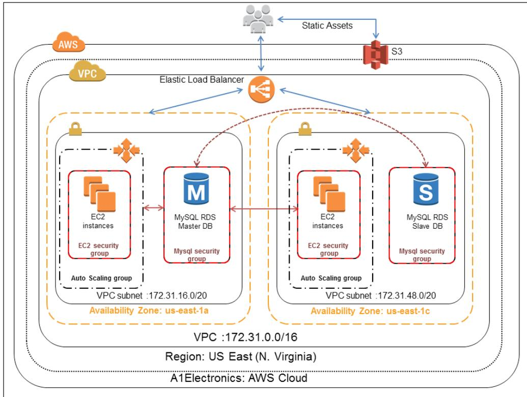
The application is hosted in the US East region of the AWS cloud. This architecture is designed to handle failures within a region and not across regions.
