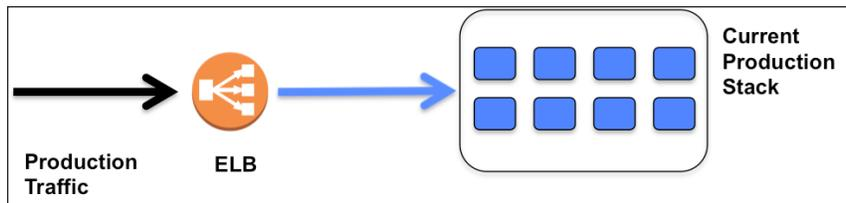
2. In this stage, you create a new instance hosting the new stack (in a separate auto scaling group with a max size of 1). While the blue fleet is serving a majority of production traffic, the green instance also starts serving some of the production traffic.
