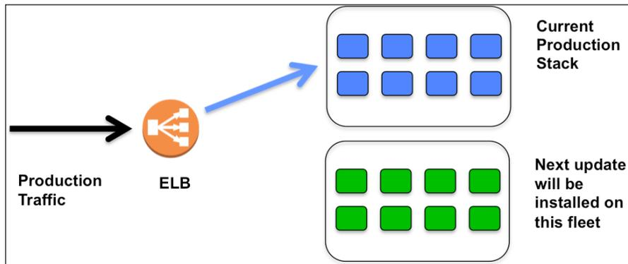
The primary advantage of the blue-green approach is that you are not touching the currently running stack at all. You also have the option to fallback to the old stack at any time, easily. However, blue-green deployments are expensive, as this approach requires you to spin up a duplicate set of instances.
