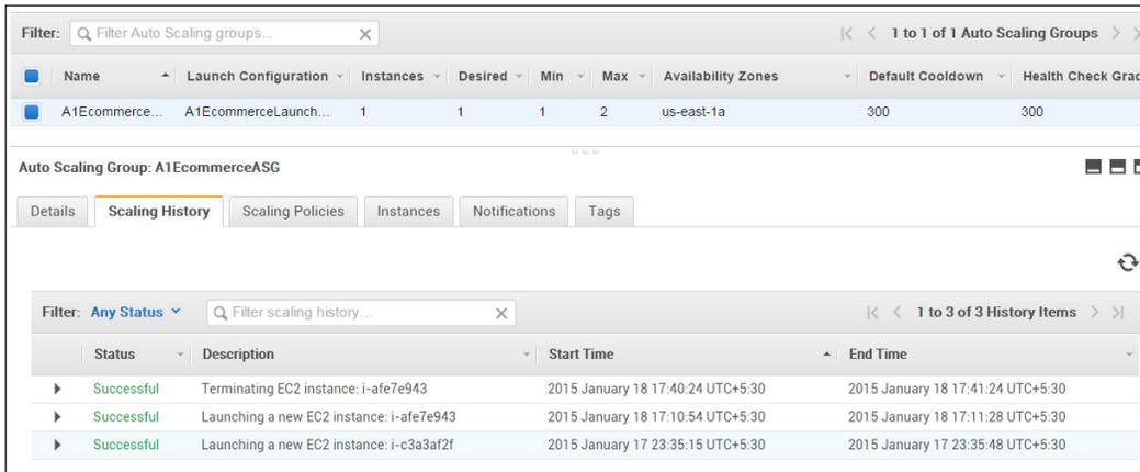
In the same way, we can verify the scaling in by the auto scaling group, that is, removal of an EC2 instance when the average CPU utilization of the EC2 instances falls below 30 percent for a period of 20 minutes. This can be achieved by ending the bc task. The average CPU utilization of the instances will fall below 30 percent and scaling in threshold will be breached after a period of 20 minutes.
