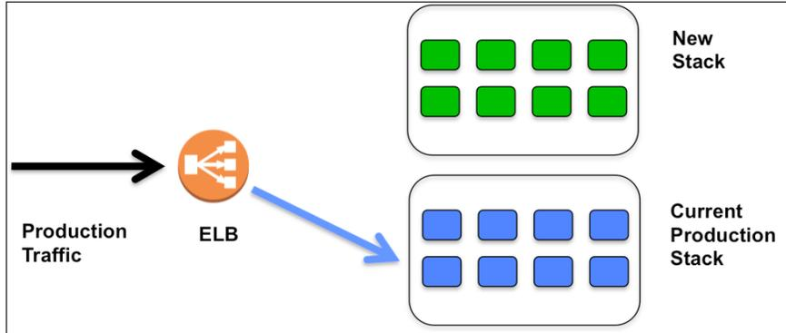
2. Verification and acceptance tests for the new stack are conducted on the green fleet, while the blue fleet continues to serve the production traffic.
