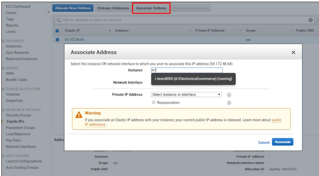
The screenshot displays the AWS Management Console interface for associating an Elastic IP address. The 'Associate Address' dialog box is open, showing the following details:
