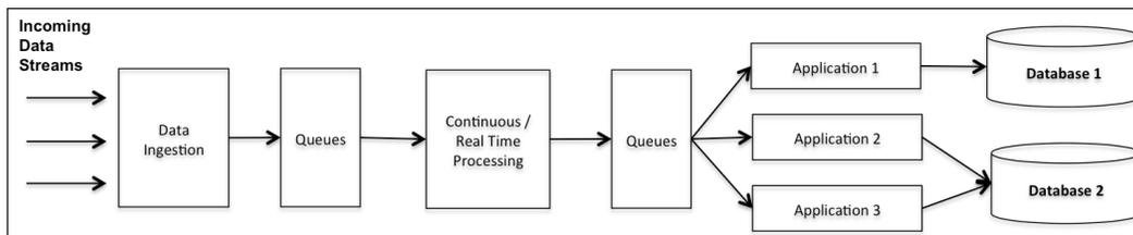
Typically, the web tier writes messages or work requests to a queue. A component from the services tier then picks up this request from the queue and processes it. This ensures faster response times for end users as the queue-based asynchronous processing model does not block on responses.
