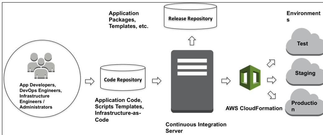
CloudFormation is a key part of your DevOps pipeline enabling faster production releases. For example, as shown in the figure, you can setup a continuous integration environment that builds your application, packages the application code and CloudFormation templates, and then uses CloudFormation templates to create the stack and deploy your application (in various environments including the final promotion to production).
