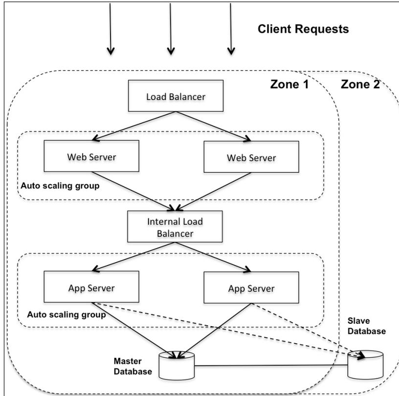
It is also possible to separate the tiers across two different regions, to provide for higher level of redundancy including data center wide or zone level failures. While designing high availability architectures across multiple regions, we need to address network traffic flow and data synchronization issues between the regions. Such issues are discussed in more detail in *Chapter 5, Designing for and Implementing High Availability*. The following diagram illustrates this architecture:
