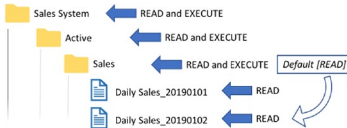
Figure 5-6. Default permissions are configured on the “Sales” folder to allow for a new file to be accessed by a principal
