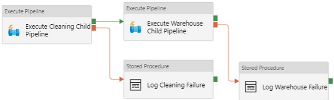
Figure 3-25. An image of single error handling activities being hooked to the “On Failure” outputs of Execute Pipeline activities, avoiding the need for duplicated error activities
